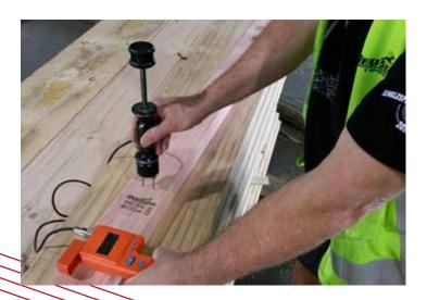
Measuring Moisture in radiata pine using a meter with long insulated prongs: Hammer 1/3 the way through the piece and at least 600mm from the end. Make sure batteries are fresh, meter is calibrated correctly and a correction is applied for species and treatment. For additional technical information about Red Stag Timber Products ask your merchant to arrange a training program with their Red Stag Timber professional
