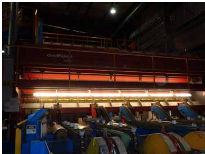
GradExpert: Optically grades for visual consistency and removes boards that fail to comply with this specification
