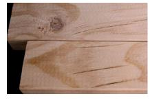
**CHECKING:** Is the term used for surface wood cell separation sometimes inherent in the log but can be worsened by aggressive kiln drying. It can lead to splitting.
