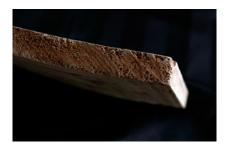
**CUPPING:** Can be caused by a moisture gradient between the timber faces or by differences in the timber density through the piece which results in differential shrinkage during drying.
