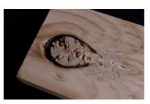
**BARK ENCASED KNOT:** Occurs where there is minimal connection between the knot and the surrounding wood fibre.
