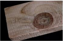
**INTERGROWN KNOT:** Occurs where there is strong connection between the knot and the surrounding wood fibre.
