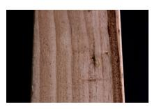
**PITH:** Is the dead cell structure at the very centre of the log. It indicates the centre of the corewood area and timber sourced from this region is lower density, has lower structural properties and is prone to distortion because of the angular grain.
