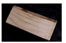
**WANE:** A board coming from the outside of the log has the best mechanical properties and can sometimes be identified by the curved portion along the edge.
