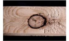
**LOOSE KNOT:** Occurs where there is no connection between the knot and the surrounding wood fibre.
