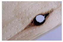
**HOLE:** A Hole is where a loose knot has fallen out. Structurally, a hole is considered no differently from a knot.
