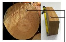
**COMPRESSION WOOD:** A tree with constant stress in one direction (wind or gravity) may develop compression wood to compensate for the force. This wood fibre has different cell structure indicated by the dark bands and is likely to be prone to distortion.
