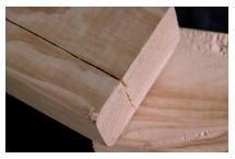
**SPLITTING:** Results near the end of a board, aggravated by aggressive kiln drying and further by rough handling, poor moisture control and mechanical force (e.g. strapping in the packet).
