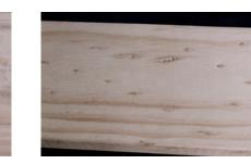
**NEEDLE FLECK:** Is the term used to describe pine needles that have become encased in the log as it grows in diameter. It is a visual defect but does not affect the mechanical properties of the timber.
