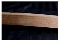
**CROOK:** Is distortion in the direction of a joist. It can be caused by moisture differential through the piece or by corewood on one edge leading to uneven shrinkage during drying.
