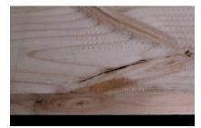
**DOUBLE SPIKE KNOT:** Is where a spike knot enters the board from either edge in the same area of the board. The resulting grain deviation is likely to reduce mechanical properties in that area.
