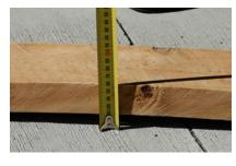
**BOW:** is distortion in the direction of a plank. It can be caused by moisture differential through the thickness or by a mix of corewood on one side and leading to uneven shrinkage during drying.
